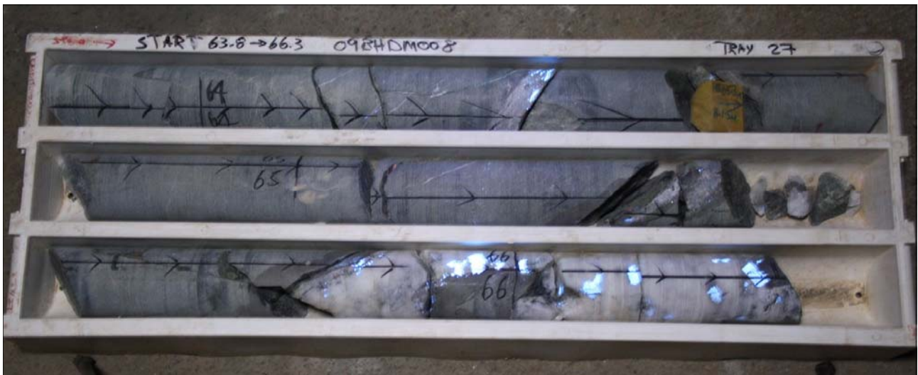
Coarse scheelite in metallurgical core from the Big Hill Tungsten Deposit . Oriented PQ diameter core.
