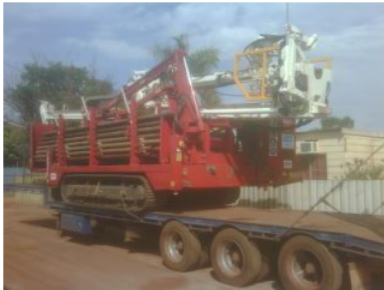
Colby Drilling's Fraste FS250 core drilling rig - one of several rigs to be utilised in a major drilling program at the Cookes Creek Tungsten Project
