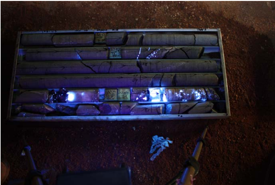
Coarse scheelite in hole 09BHD018 - oriented HQ core
