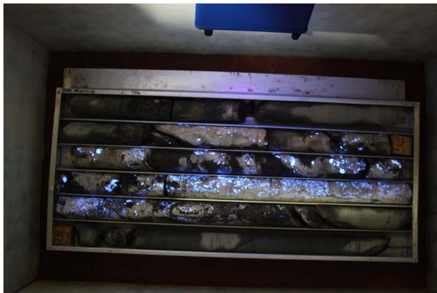
Coarse scheelite in hole 09BHD033 - unoriented HQ core
