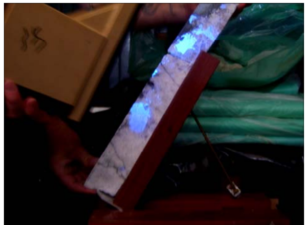
Coarse scheelite in 08BHD001 at 89m down-hole
